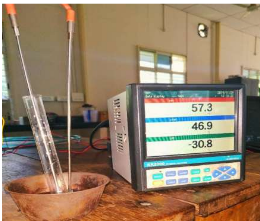
Fig. 4: Data logger used for estimating the paraffin characteristics
