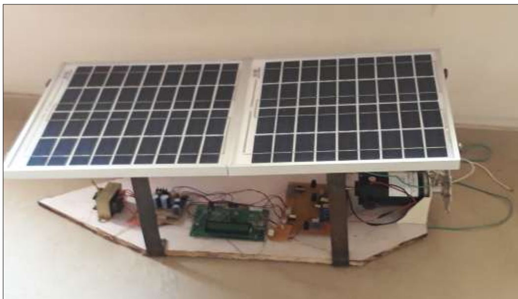
Figure 15: Hardware Implementation of the Photo Voltaic Powered Sailing Boat
