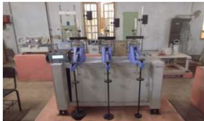
Fig. 2: Odeometer test in progress
