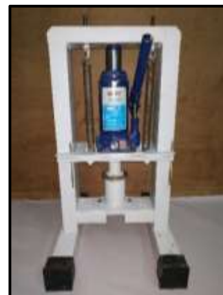
Fig. 2: Picture of Hydraulic Compressor used for disc preparation
