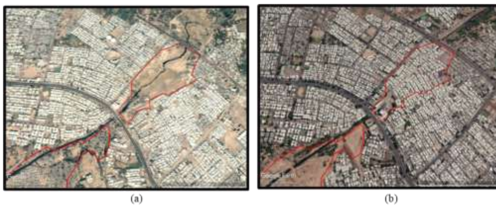
Fig. 10: Construction on rivulet flood plain at Varasiya (a) 2000 (b) 2019
