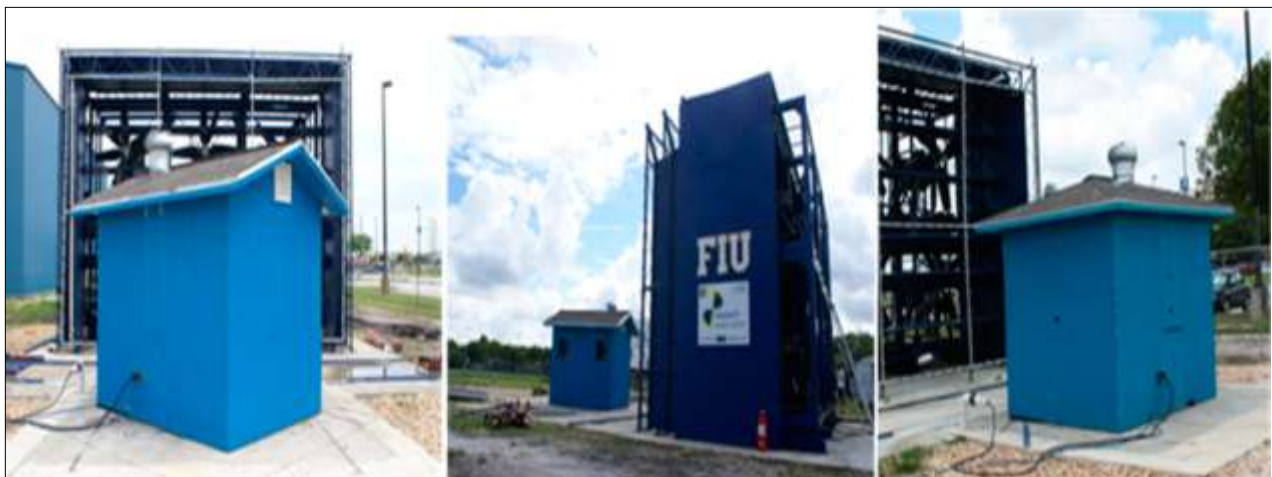
Fig. 2: Low-rise building with a gable and a hip roof in front of WOW in a testing position 99
