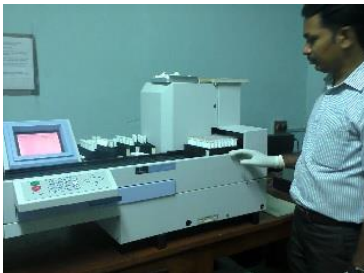
Figure 5: Melatonin Assay by RIA counted in a gamma counter from Automatic Gamma Counter (1480-11 Wizard 3), Perkin Elmer, USA.
