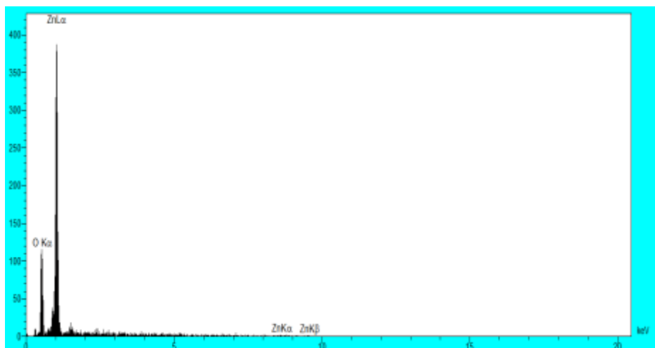
Figure 6: EDS Spectrum of Synthesized ZnO Nanoparticles
