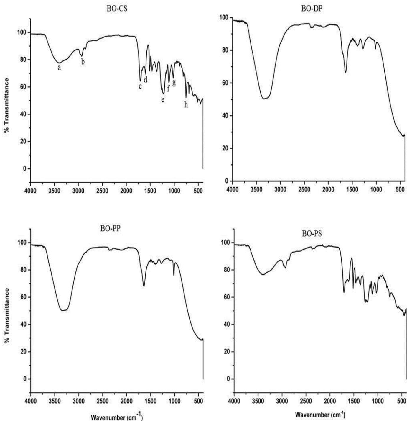
Fig. 3: FTIR spectra of the bio-oils from various agricultural residues.
