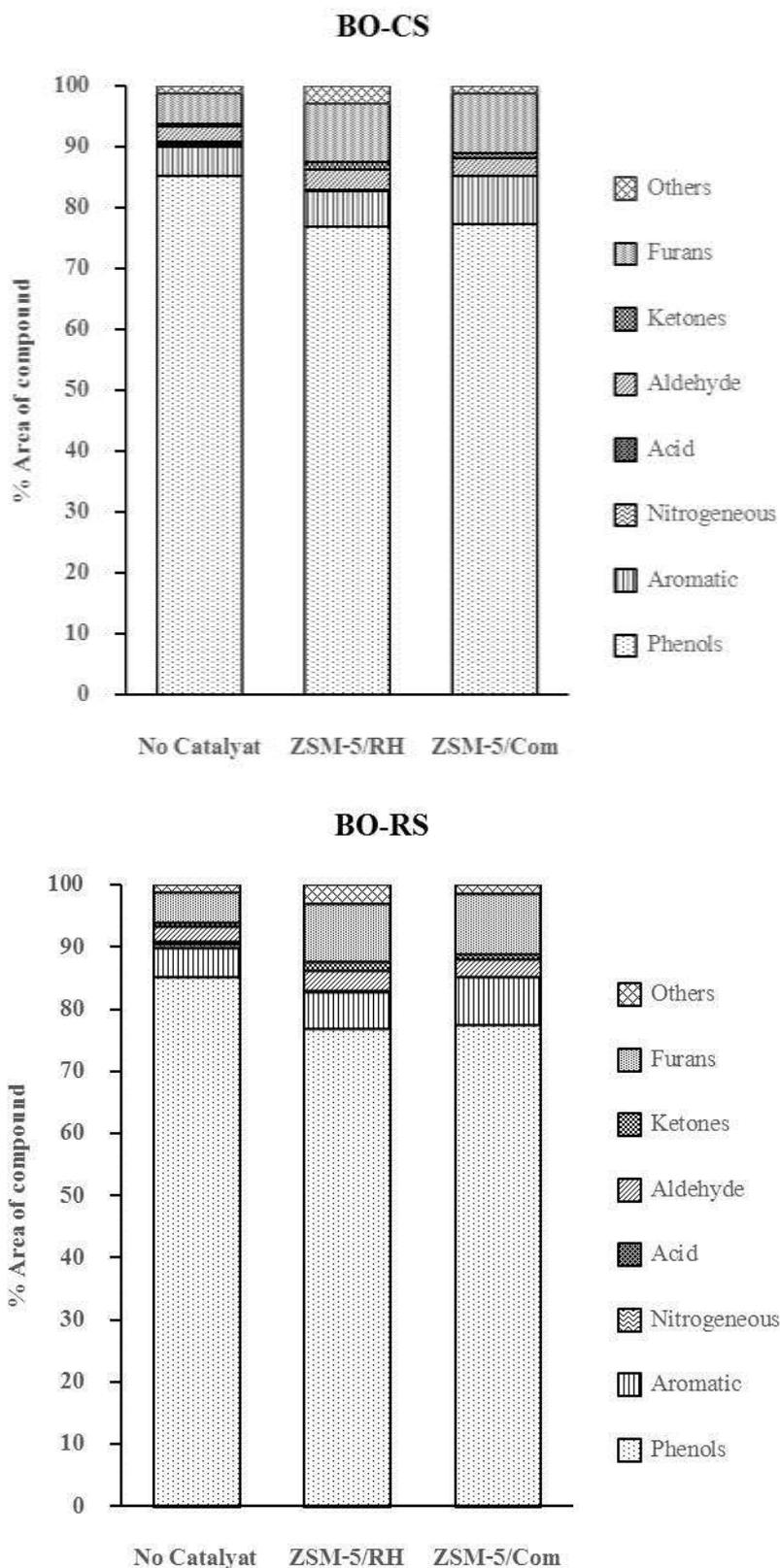
**Fig. 4: Bio-oil compositions of BO-CS and BO-RS obtained from various pyrolysis systems**
