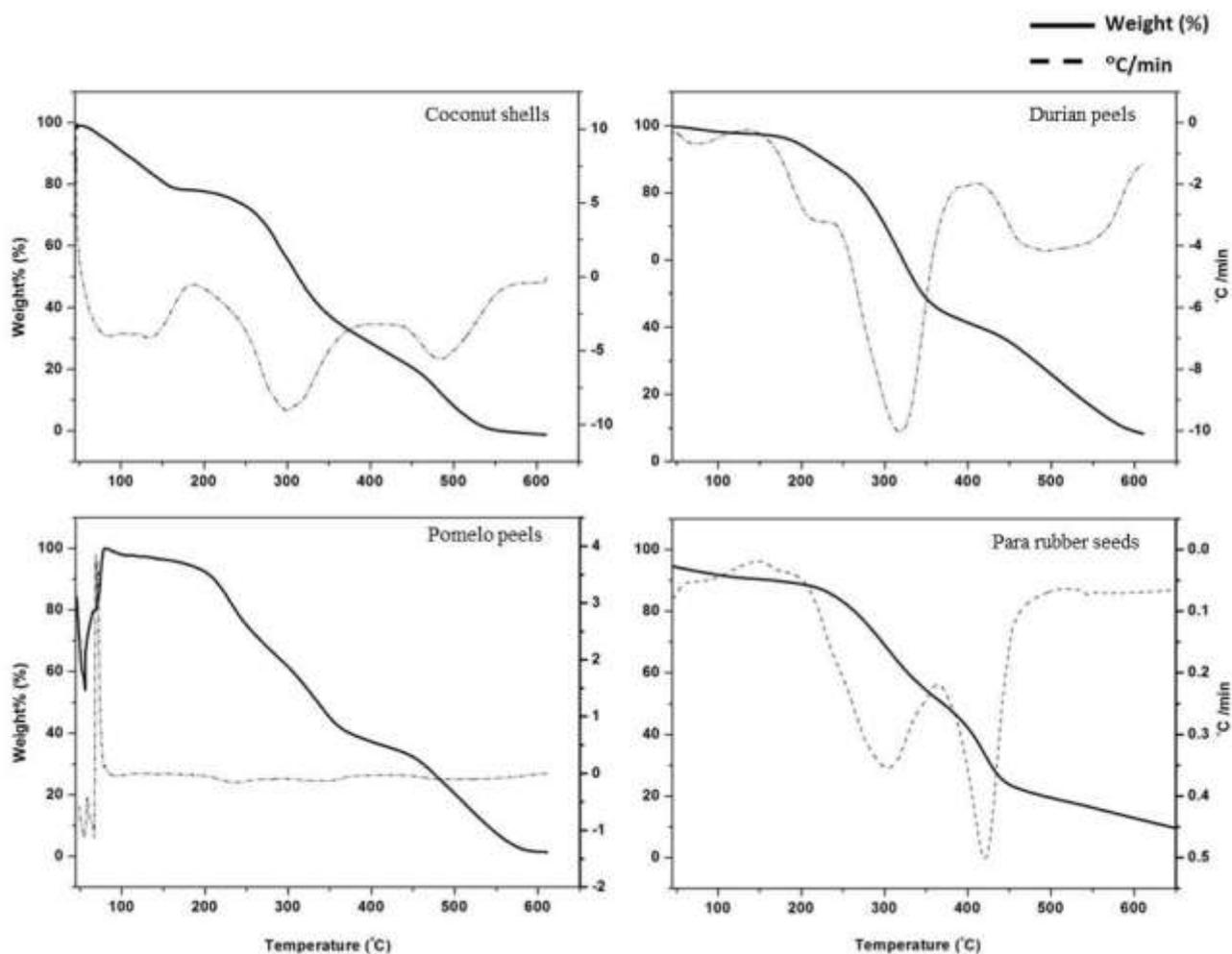
Fig. 1: TGA and DTA profiles of the agricultural residues
