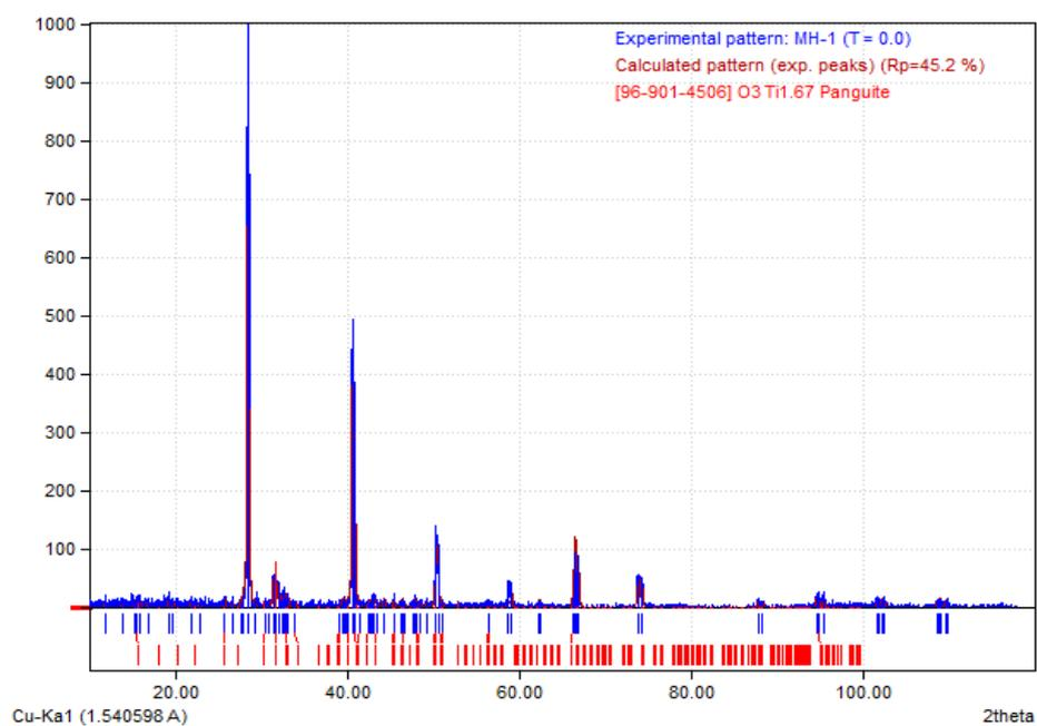
Fig. 2: XRD Spectra of TiO<sub>2</sub> NPs
