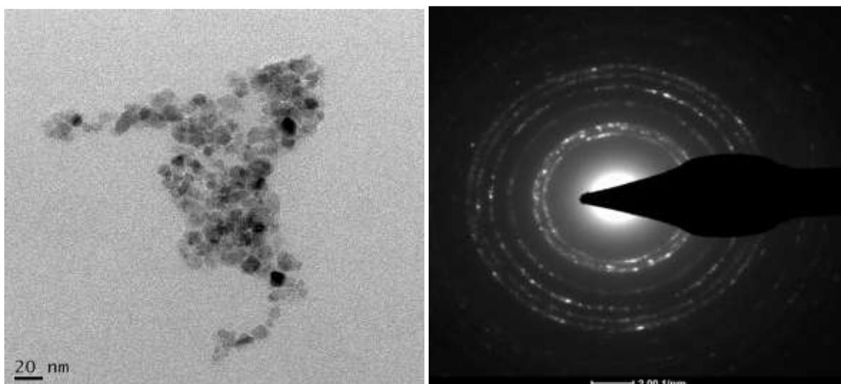
Fig. 4: TEM image and SEAD image of TiO<sub>2</sub> NPs
