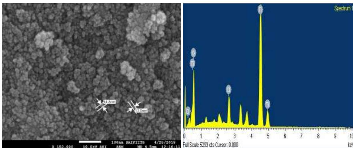
Fig. 3: SEM and EDX Spectra of TiO<sub>2</sub> NPs
