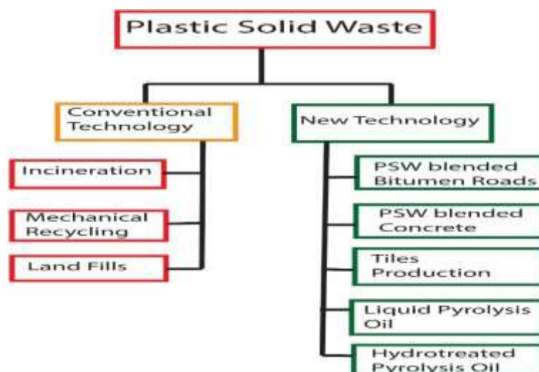
Fig. 1: Technologies for disposal of PSW
