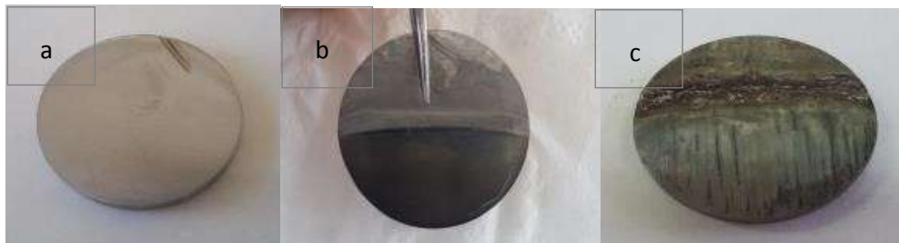
Fig. 1: Metal alloys Ti-6Al-4V (a) before anodization (b) anodized product with DC current and (c) anodized product with AC current
